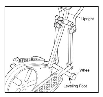
If the elliptical exerciser rocks slightly on your floor, turn one or both of the leveling feet under the front stabilizer until the rocking motion is eliminated.
